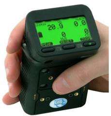
Exposing the instrument to known concentration test gas verifies that gas is properly able to reach and be detected by the sensors. It verifies the proper performance of the instrument's alarms, and (if the instrument is equipped with a real-time display), that the readings are accurate.
