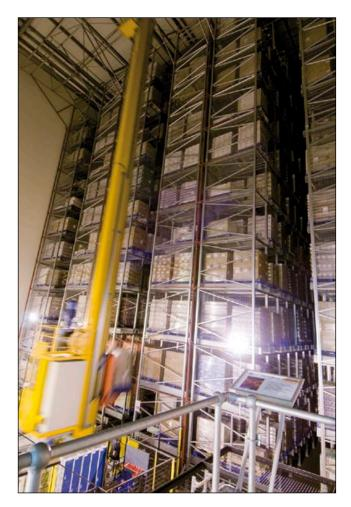
**Figure 19** An automated narrow aisle fork-lift truck in operation
