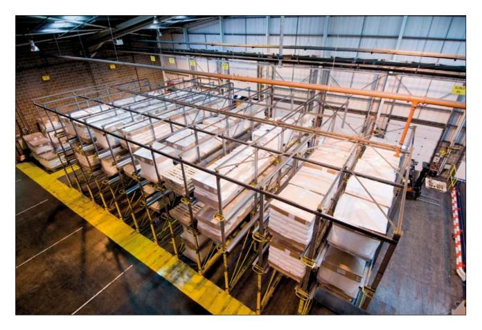
**Figure 15** Storage of packaged dangerous goods in racking
