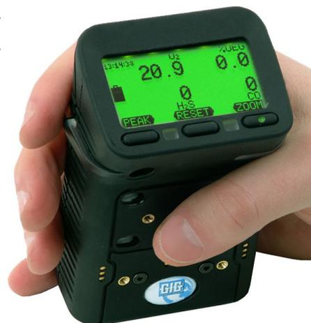
This functional "bump test" is very simple and takes only a few seconds to accomplish. It is not necessary to make a calibration adjustment unless the readings are found to be inaccurate. The regulatory standards that govern confined space entry and other activities that include the use of direct reading instruments are in agreement with this approach.
