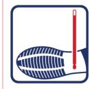
HRO - Heat resistance of the outsole. Resistance to a short term hot contact with the outsole up to 300°C for 1 minute. The sole will not be damaged
